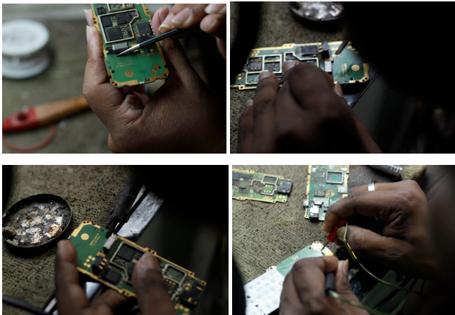
Figure 2: Steps of jumpering (clockwise, from top-left): Showing the broken audio connection, Reconnecting two points with a piece of wire, Melting wire with soldering iron, Rechecking the connection.
